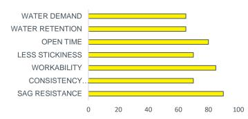
Chemical base: Viscosity: Particle size: Moisture content: Cellulose ether derivate (HPMC) Approximately 10.000-20.000 mps Fine powder Max 8%
